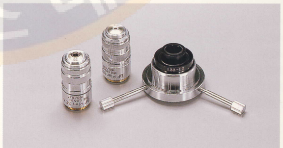
Darkfield condenser and objectives with iris diaphragm
